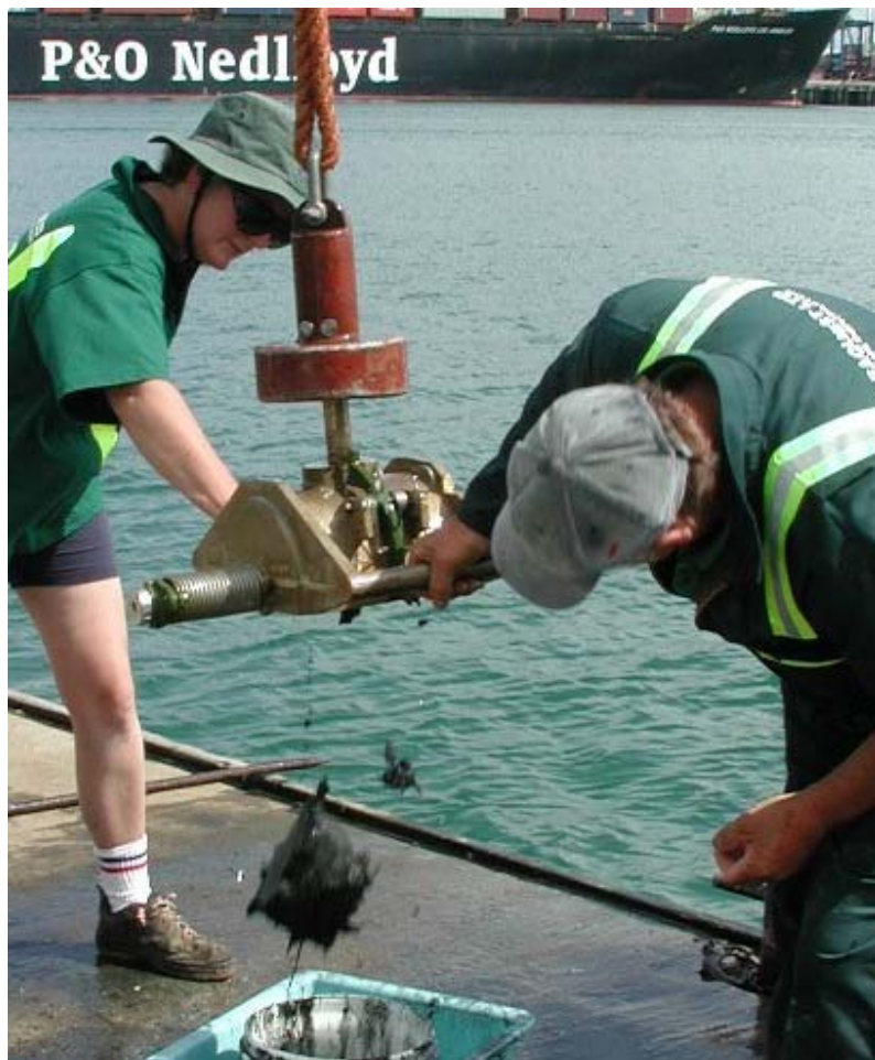
Figure 4: Shipek grab sampler: releasing benthic sample into bucket
