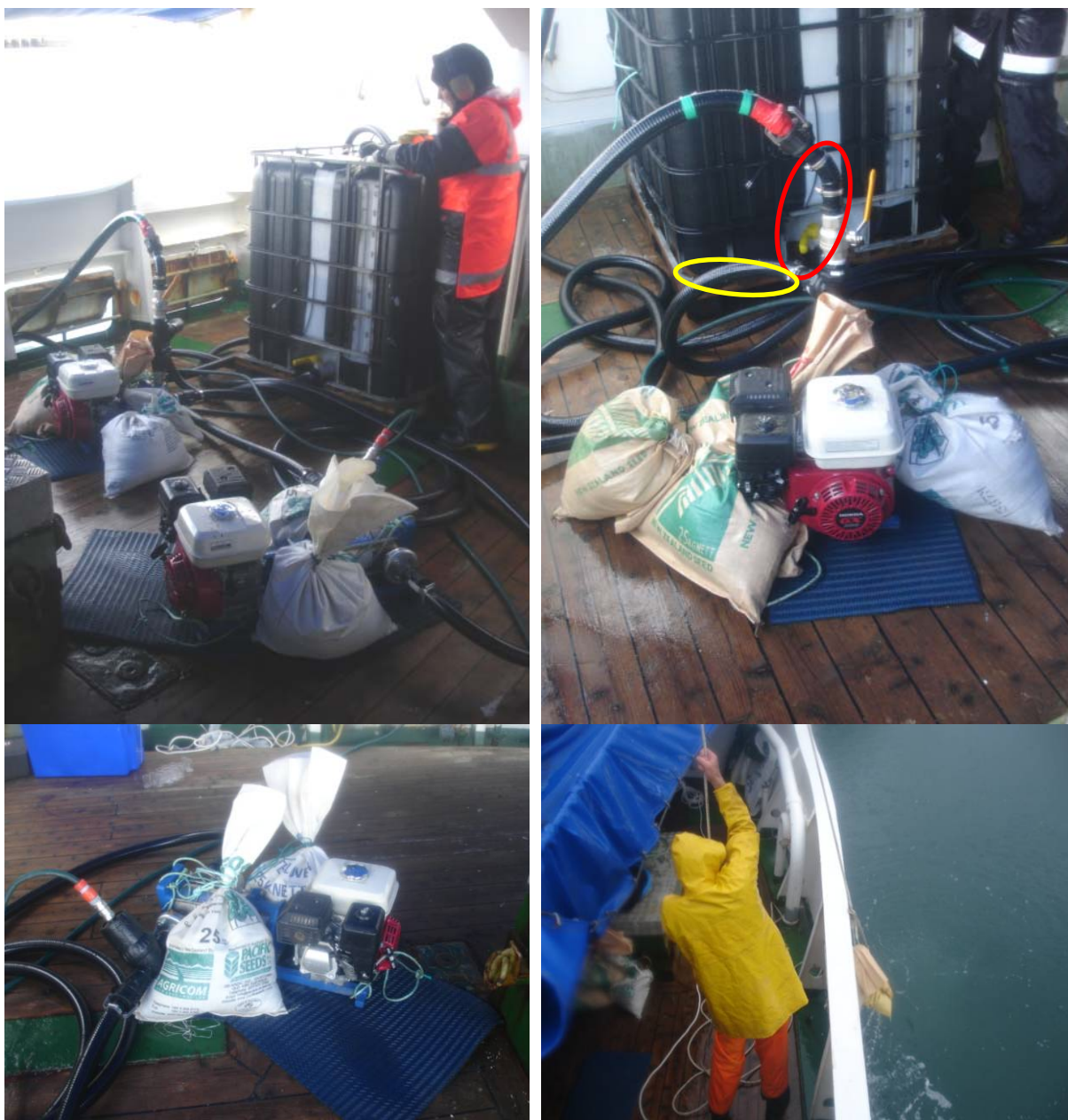
Figure 2.10: IBC header tank, pumps and hoses established on the vessel (top left). Lowara CO350/03 (top right) and Lowara SV205 T304 (bottom left) pumps secured to the deck. Sandbags being recovered using the ship's derrick, rope and pulley (bottom right).
