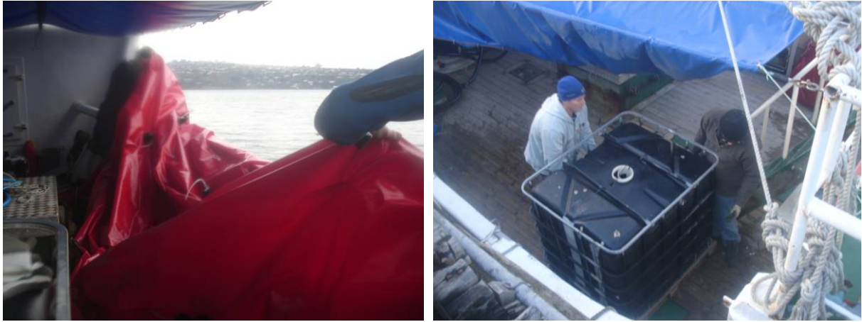
Figure 2.11: Deployment of the tarpaulin over the gunwale (left). Header tank being loaded onto vessel (right).
