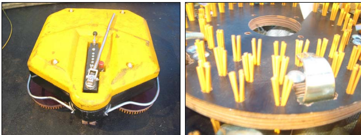
Figure 5 Sub-Sea Industries MC312 Typhoon brush cart (left) with Rislan brushes and scrapers (right)
