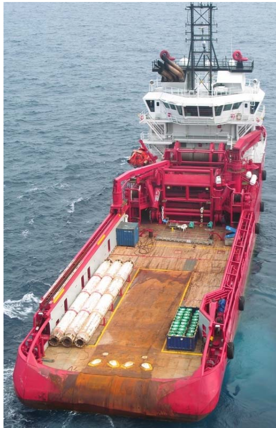
Figure 8 A typical oil rig supply vessel which has sufficient beam to accommodate the IMProtector across its work deck and tank capacity for collecting treatment waste water
