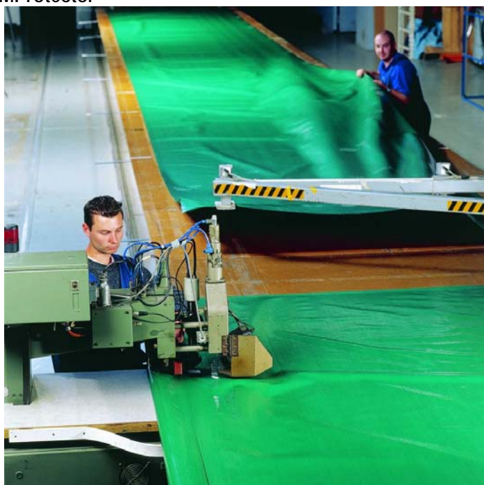
Figure 21 The bunker cover manufacturing table in Bartlett's factory which could be used to build a 1/3 scale IMProtector
