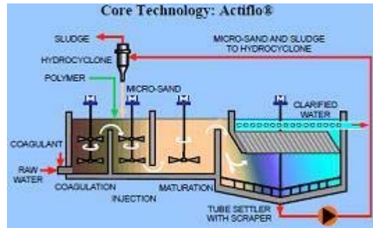
Figure 12 AHCS Treatment System Diagram
