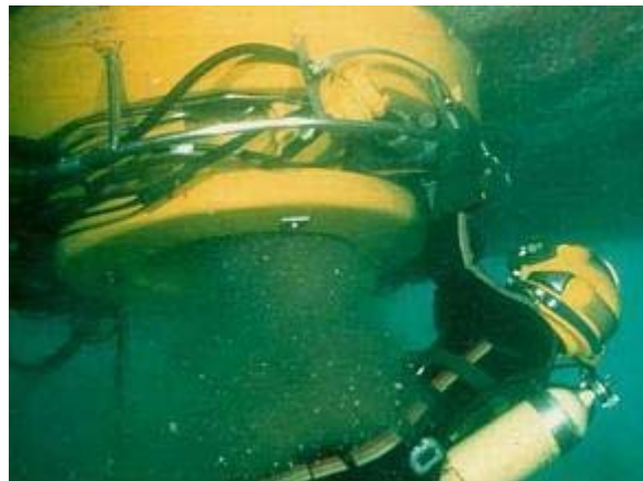
Figure 7 Scamp hull cleaning showing discharge of marine fouling
