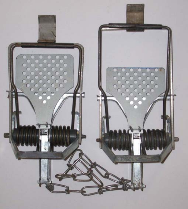
Figure 5: Original (left) and modified (jaws extended 35 mm and trigger plate shortened by 15 mm) (right) Holden Multi Kill trap.
