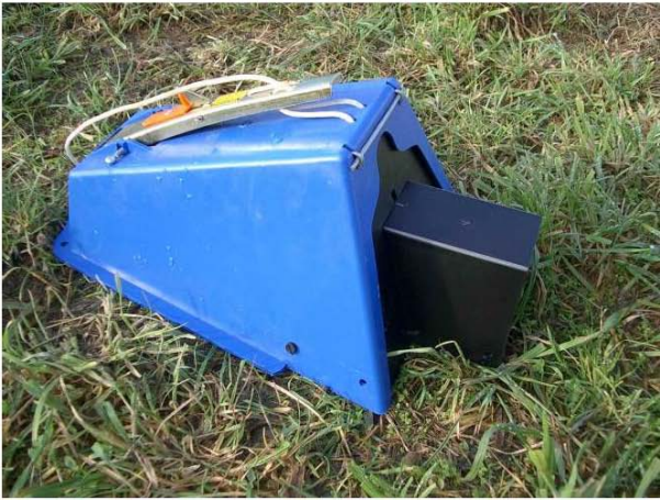
Figure 2: Sentinel trap showing plastic bait holder on trigger plate (left) and with Corflute® cover (right).
