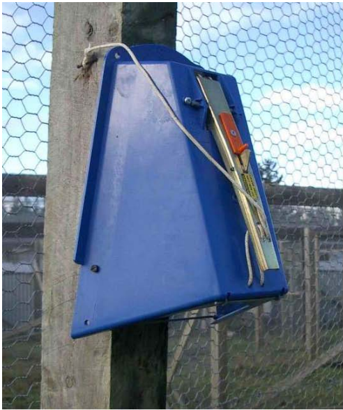
Figure 1: Possum Master trap set for possums (left) and ferrets (right). This trap is the only commercially available kill trap in New Zealand that uses a string noose as the killing mechanism.
