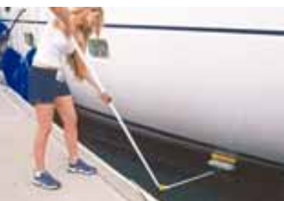
CLEANING THE SLIME LAYER BY REGULAR BRUSHING OF THE HULL
