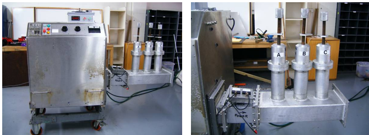
Figure 3: a) Five kW Microwave generator, and b) three-stub impedance tuner (labelled A, B, C) on waveguide with waveguide dual directional coupler.
