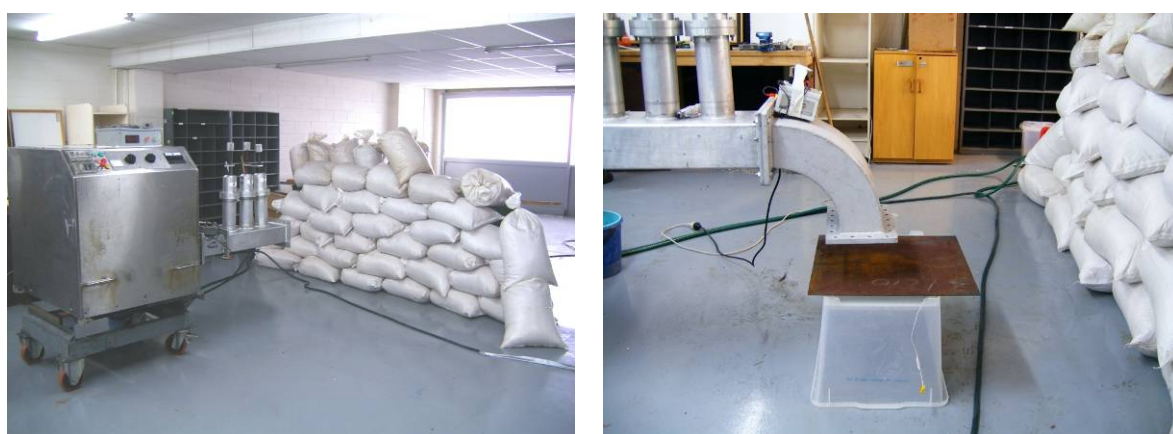
Figure 4: a) Screen of sawdust bags, and b) Elbow attachment to treat horizontal surfaces.
