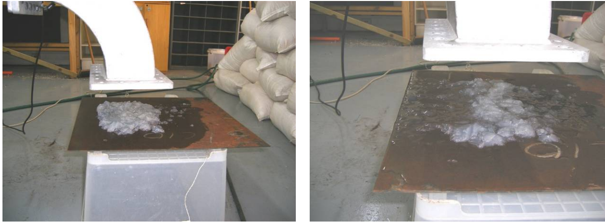
Figure 8: a) Gelatine layer on a horizontal surface before heating, and b) after heating.
