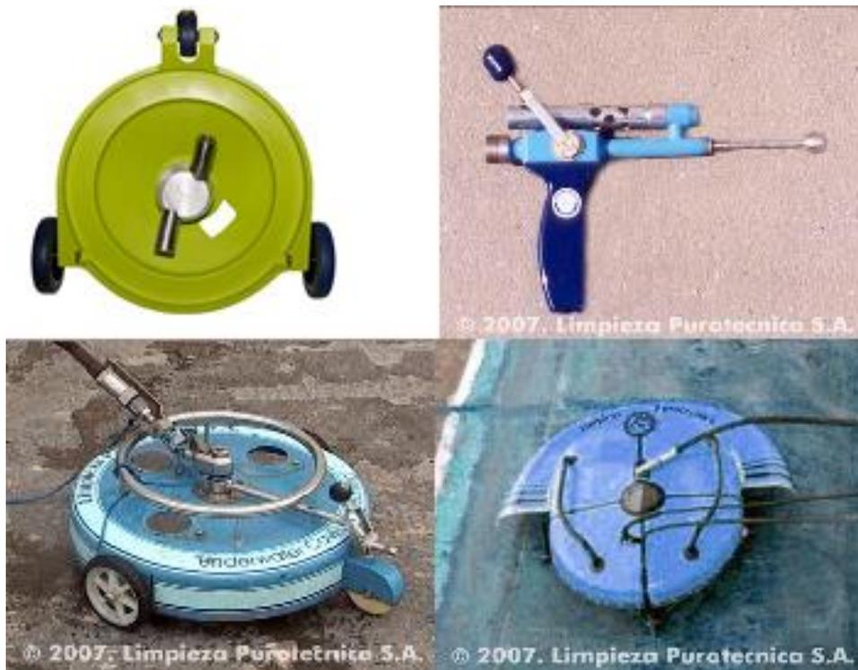
**Figure 8: Examples of cavitation-jet cleaning equipment.**
