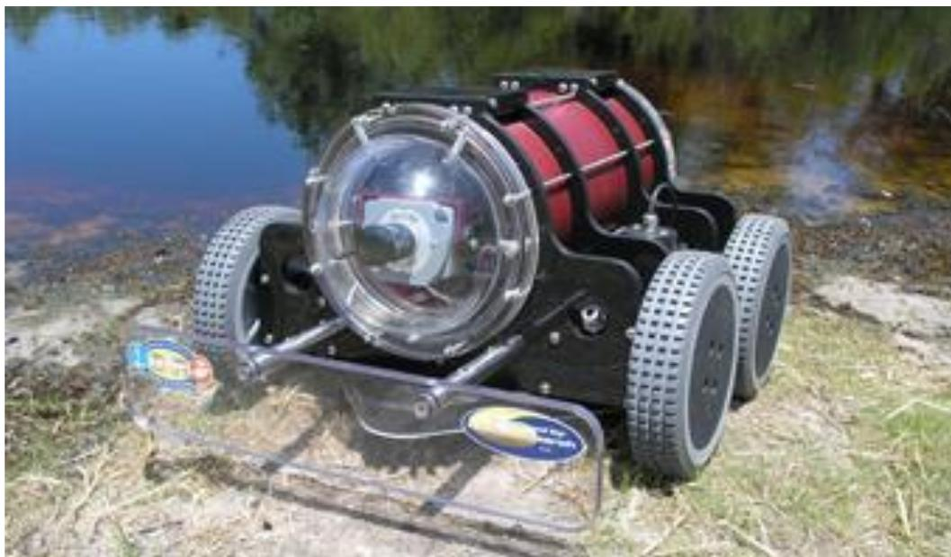
**Figure 4: The US ONR's Hull BUG robotic cleaner.**
