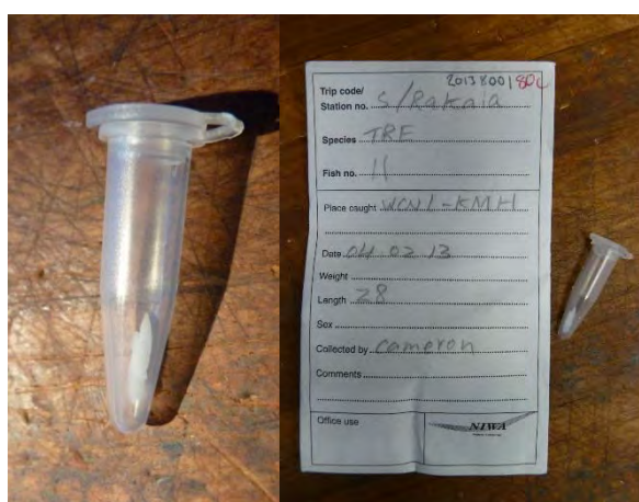
Figure 1: Images of a microcentrifuge tube and envelope used to store small and fragile otoliths like those collected from tarakihi.
