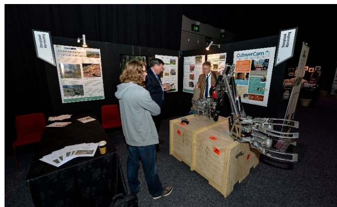
The 'Stick Insect' tree felling machine developed by the Steepland Harvesting PGP programme.
