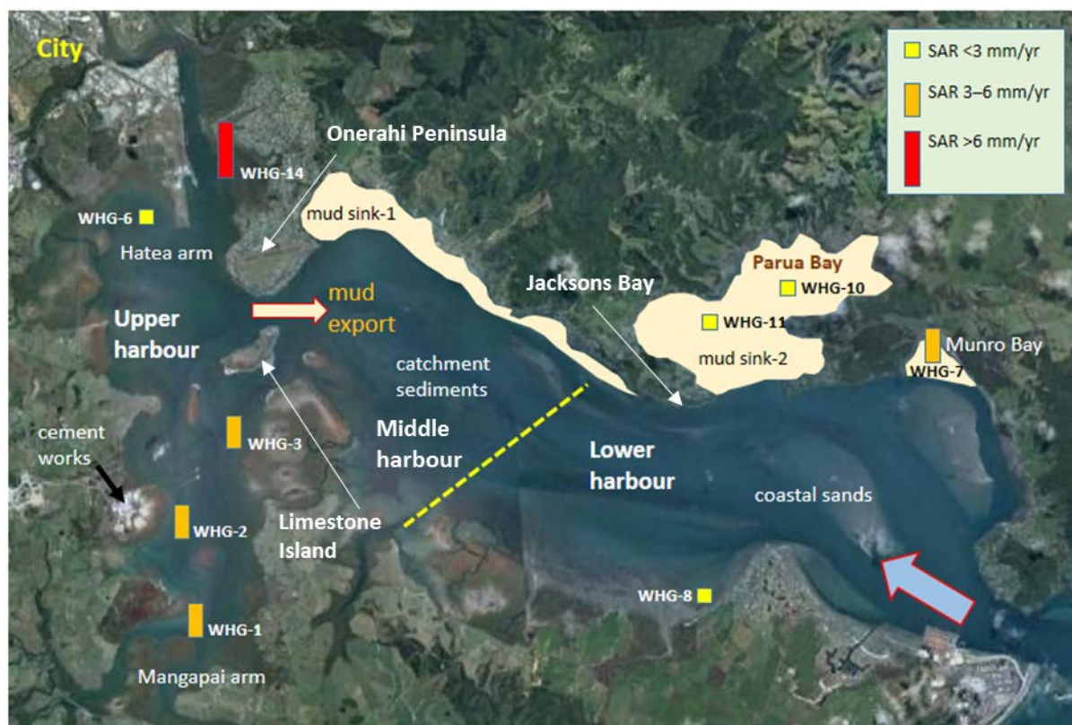
Figure 3-2: Location map, including the locations of the three long-term mud sinks east of Onerahi Peninsula identified by Swales et al. (2013). Reproduced from Swales et al. (2013). The light yellow areas showing the mud sinks correspond to (from west to east) the NS , PB and MB depositional basins in the harbour sediment budget.
