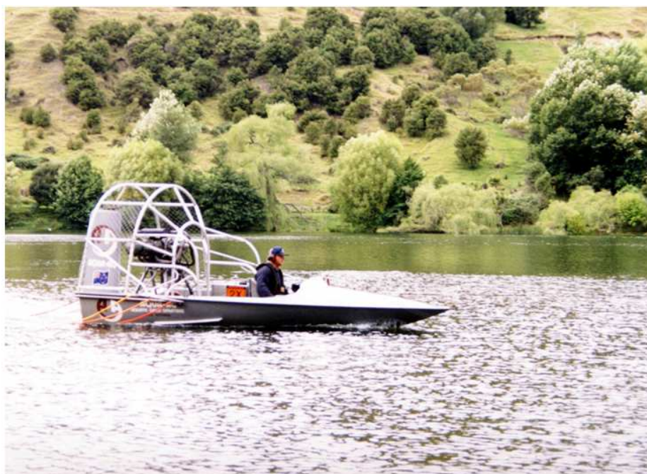
Figure 8: An airboat (Aqua-Ag) dispensing herbicide with weighted trailing hoses.
