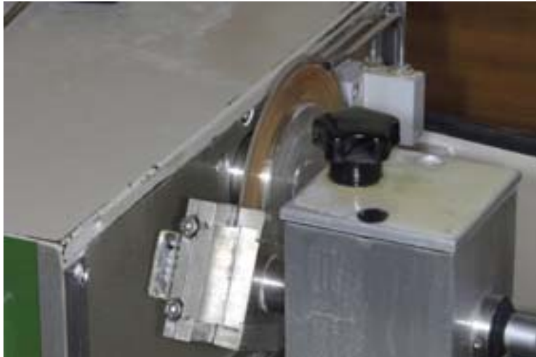
Struers Accutom-2 saw with twin wafering blade set up.
