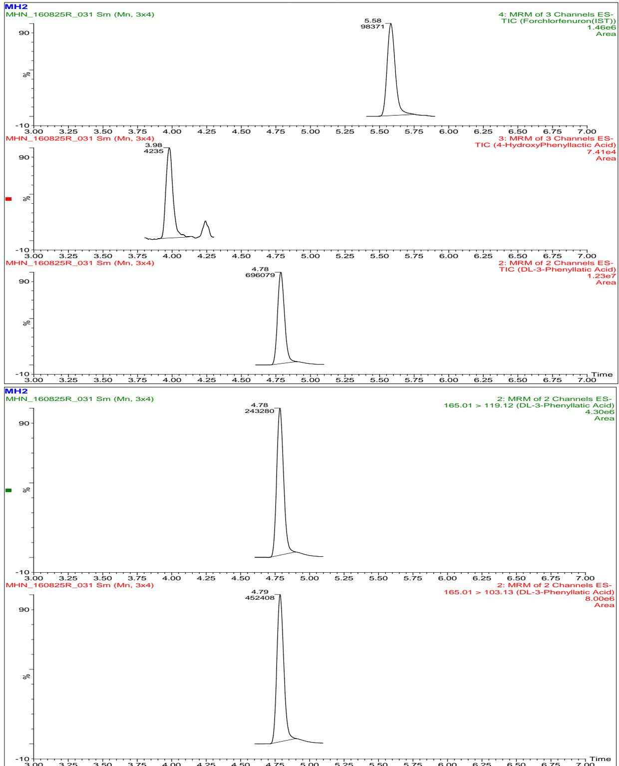
**Figure 7: MRM of 2 Channels ES- for 3-phenyllactic acid of 1.0 mg/kg honey spike and 0.05 mg/kg matrix standard**
