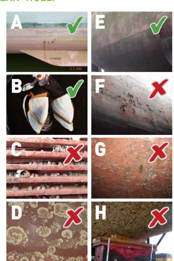
The only fouling a long-stay vessel may have is a slime layer (A) and gooseneck barnacles (B). Any other species, such as the acorn barnacle (C), or bryozoans (D), are not allowed. The images on the right show a slime layer (E) which would meet the new requirements, and moderate (F) extensive (G) and very heavy (H) levels of fouling which would not meet the new requirements.
