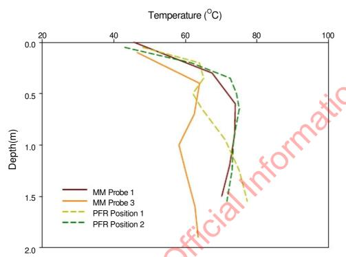
Figure 11. Vertical change in temperature (°C) at four positions in the bunker measured by Meadow Mushroom and PFR Probes.
