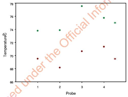
Figure 5. Mean temperatures of Meadow Mushroom probes. Green circles donate the average temperature of the stabilised cycle for each probe and red circles donate the overall average temperature. Error bars represent LSDs. Probe 1 is closest to the back of the bunker, and Probe 4 closest to the door.
