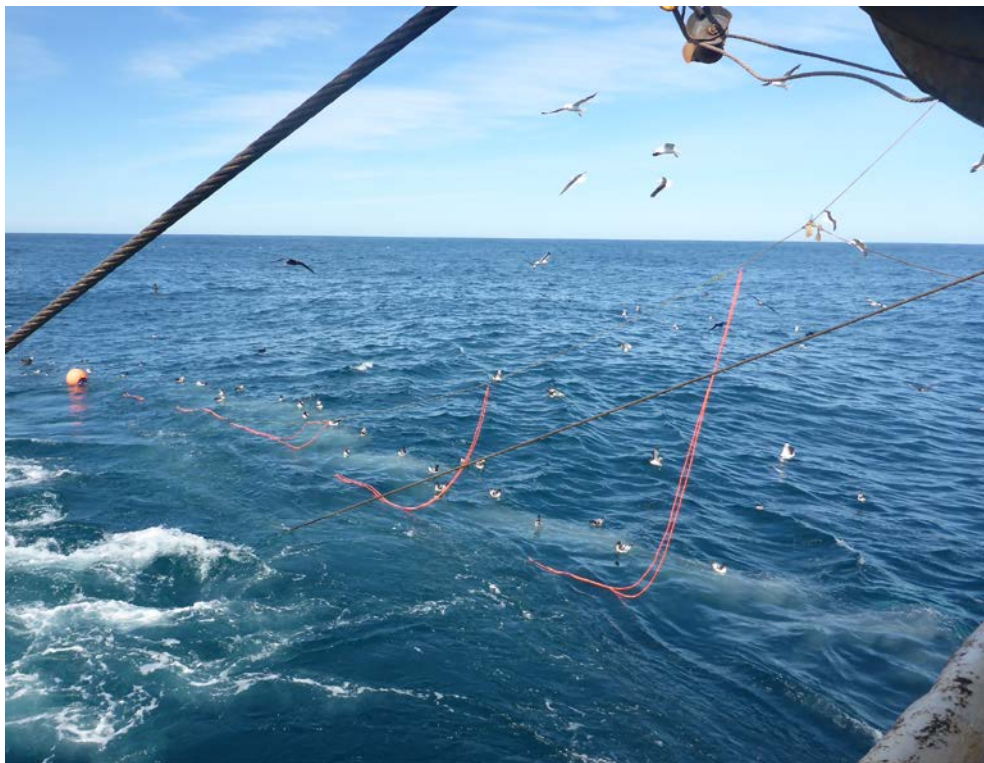
A tori line designed to prevent seabird collisions with trawl warps
