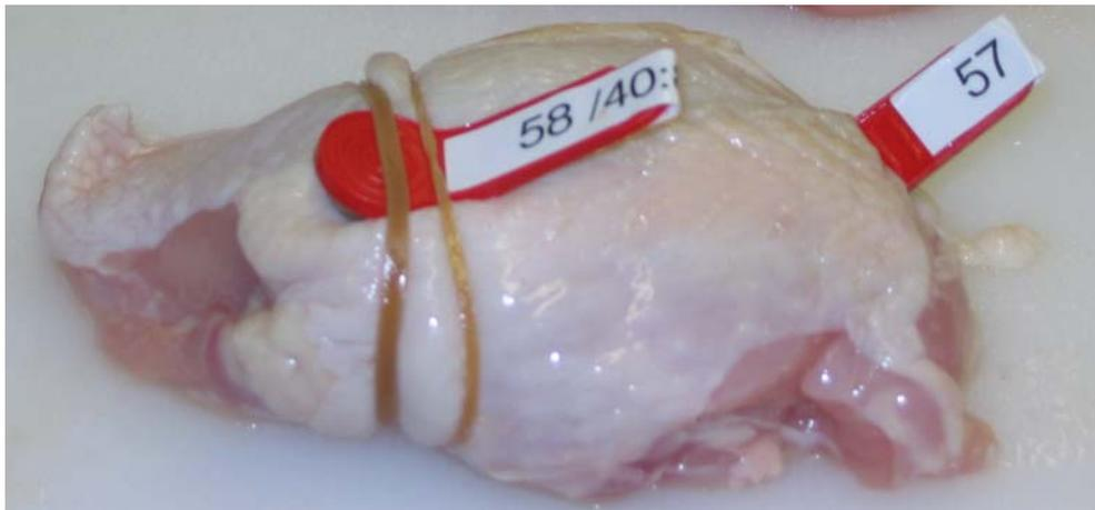
**Figure 1: Placement of internal (57) and external (58) data loggers in a skin-on breast portion**
