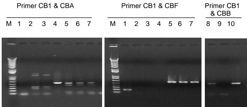
Figure 4: Specificity testing of primers CB1 & CBA, CBB, and CBF by PCR for DNA samples from colonies on blood agar sub-cultured from broth cultures at 30°C. Lanes 1–3: *C. butyricum* Type E; Lane 4: *C. botulinum* Type A; Lanes 5–7: *C. botulinum* Type F. Lanes 8–9: colonies from a contaminated broth culture of *C. botulinum* Type E beluga; Lane 10: *C. botulinum* Type 17B. M: 1 kb plus DNA ladder (Invitrogen).
