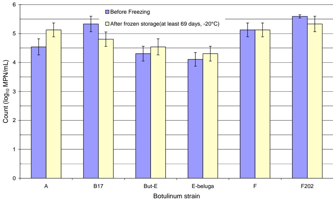
Figure 14. The effect of frozen storage (69 days at -20°C) on different BoNT-producing spores. Error bars represent standard errors of the log<sub>10</sub> MPNs.
