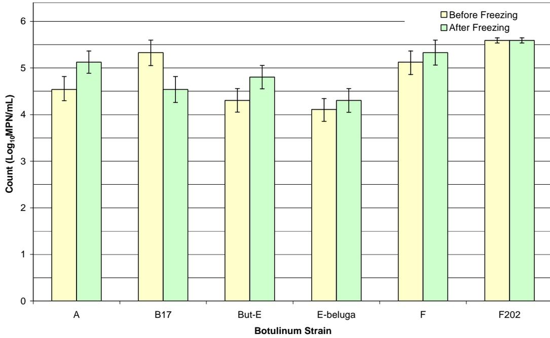
Figure 13: The effect of freezing (-85°C overnight) and thawing on different BoNT-producing spores. Error bars represent standard errors of the log<sub>10</sub> MPNs.
