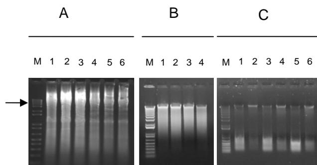
*Figure 1: Yield of DNA extraction using different approaches for C. botulinum strains grown in PYGS broth containing 10% sediment (w/v). DNA samples (5 µL each lane) were analysed by electrophoresis on 1% agarose gel. M: 1 kb plus DNA ladder with maximum molecular weight of 12 kb (arrow) (Invitrogen).*
