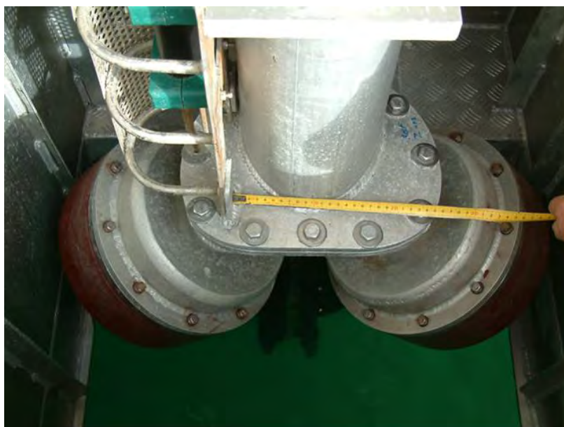
Figure 3: Multibeam echo-sounder (EM3002D) in moonpool on S.L. Ikatere . Photo by Arne Pallentin.
