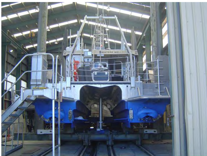
Figure 2: S.L. Ikatere from aft showing extended multibeam echo-sounder (EM3002D) pole amidships. Photo by Arne Pallentin.
