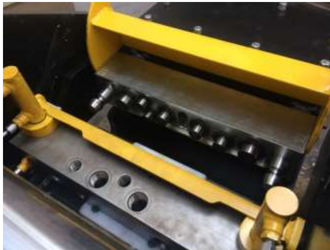
Figure 7: Close up of Doherty Quick Coupler attachment
