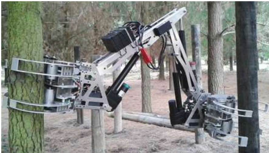
Figure 9. The robotic tree-to-tree machine at Bottle Lake Forest Park
