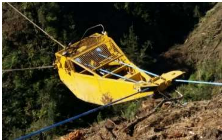
Figure 8: Prototype Skyshifter tail hold carriage
