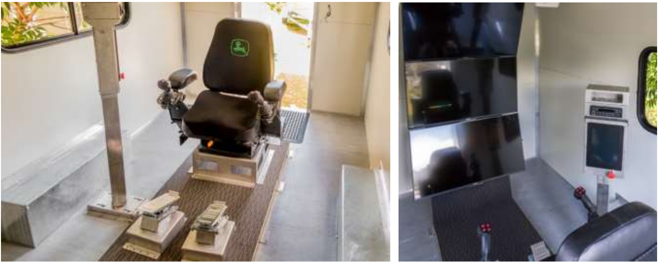
Figure 4: Full teleoperation system for John Deere 909 feller buncher
