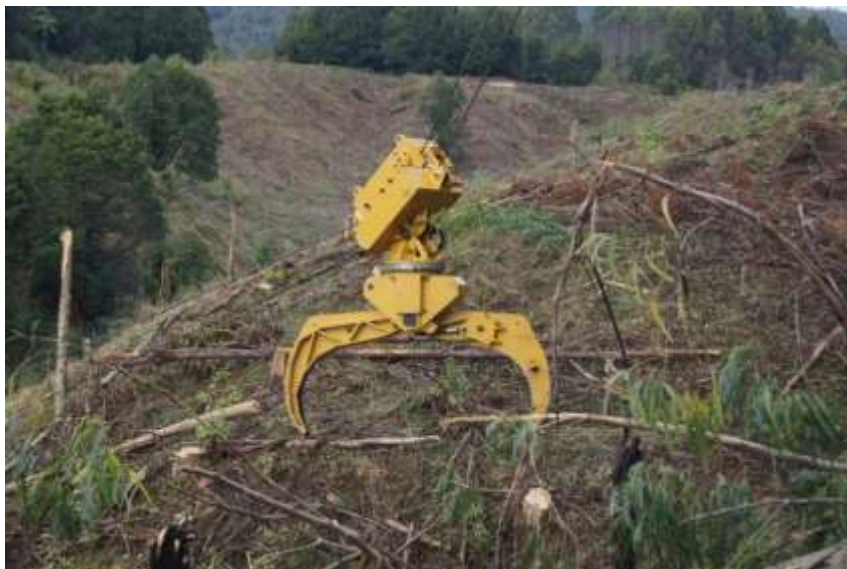
Figure 6: Commercial model Alpine Grapple Carriage
