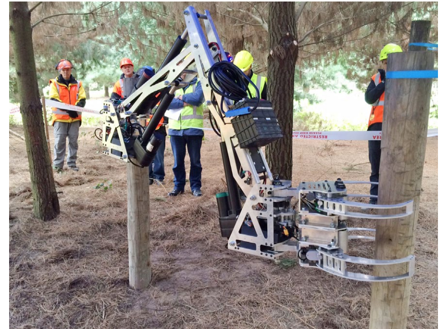
The prototype tree-to-tree felling machine developed by the Steepland Harvesting PGP programme.
