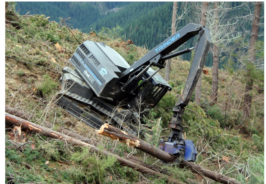
The ClimbMAX winch-assisted harvester developed by the Steepland Harvesting PGP programme.
