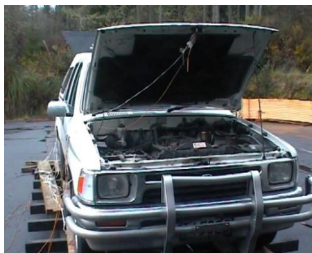
Figure 12: A vehicle undergoing heat penetration trials.
