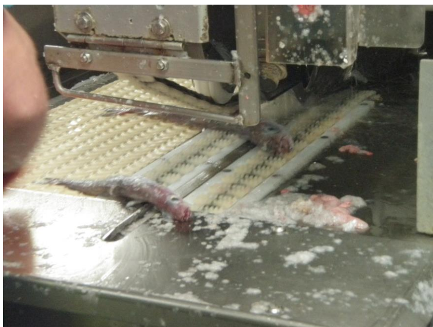
Figure 6 – Baader 424 Processing Machine – the gill plate of the fish is hooked over the alignment lug and carried through the saw by the transport belt, a secondary spring-loaded belt presses down on top of the fish as it is carried through the saw.
