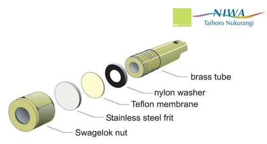
Figure 3. Exploded view of a permeation tube, taken from Lassey et al. (2001). The nylon washer was introduced into tubes filled from Dec 1998. Larger "cattle tubes" were first introduced in April 2000, prior to which two sheep tubes had been deployed in some experiments with cattle during 1999 and 2000.
