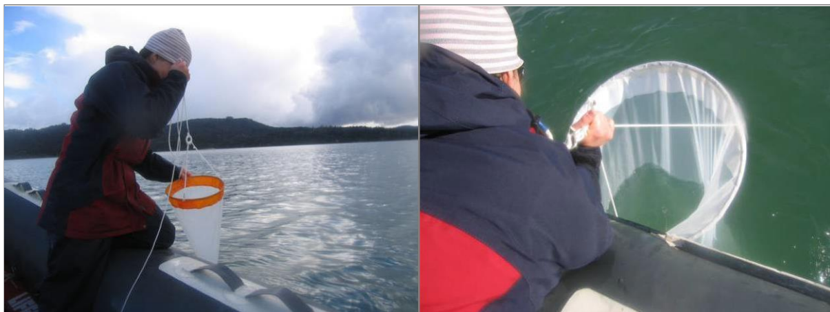
Figure 8: Field staff retrieving a plankton sample from a small net for phytoplankton (left) and a larger net for zooplankton (right).
