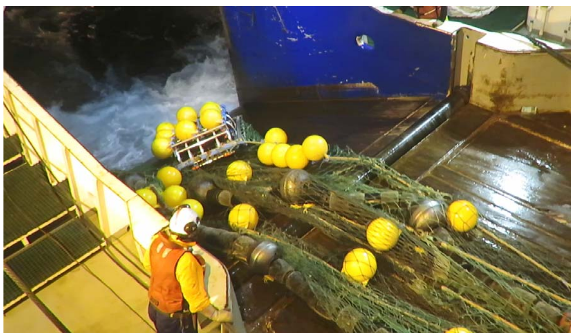
Figure 16: NIWA AOS mounted in the hoki trawl being deployed from Tangaroa (Photo by Richard O'Driscoll, NIWA).
