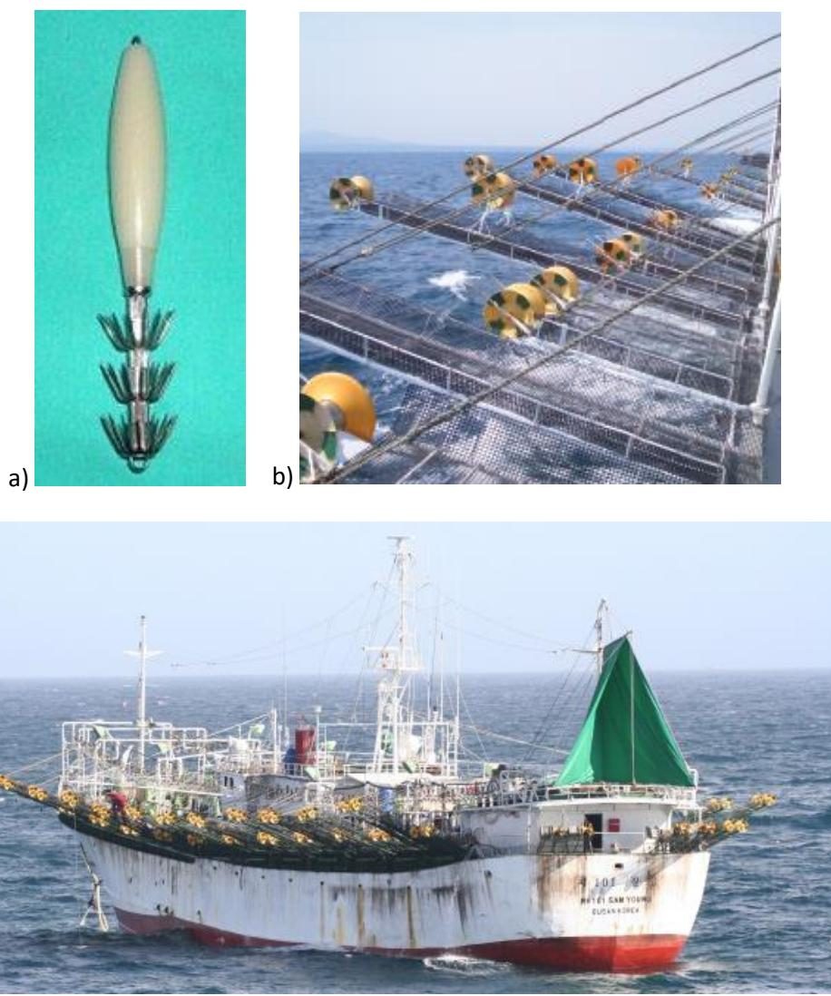
*Figure 1: a) Squid jig (Sharnbrook Tackle, 2018); b) Automated hauling blocs (PRO Japan, 2016); c) Large scale squid jig vessel (Yates, 2005).*
