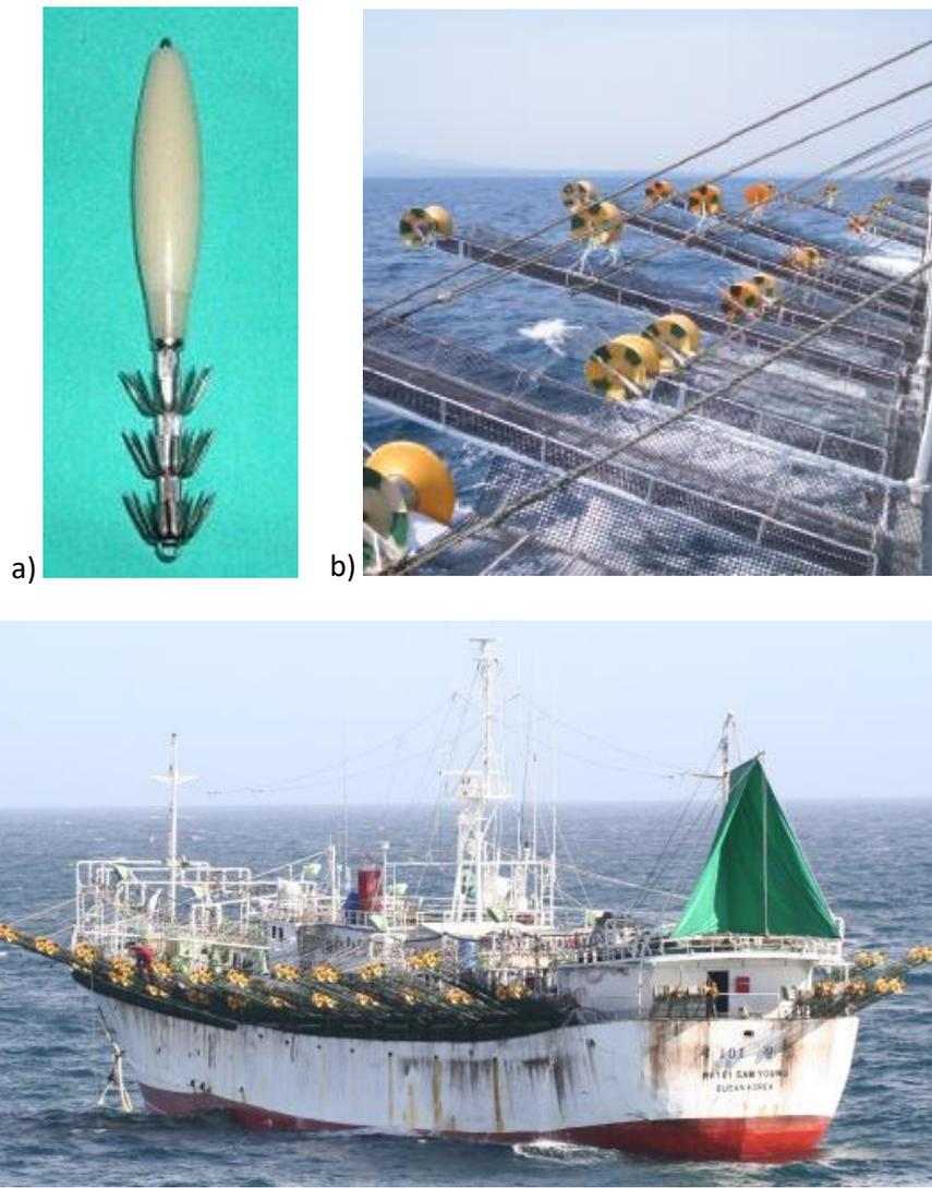
Figure 1: a) Squid jig (Sharnbrook Tackle, 2018); b) Automated hauling blocs (PRO Japan, 2016); c) Large scale squid jig vessel (Yates, 2005).
