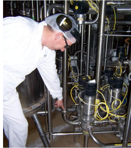
Flexihose connected for transfer from chiller to MF Line
