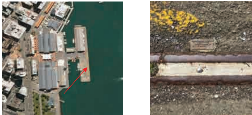
Figure 3: DD8U Mark Used for Position Check
