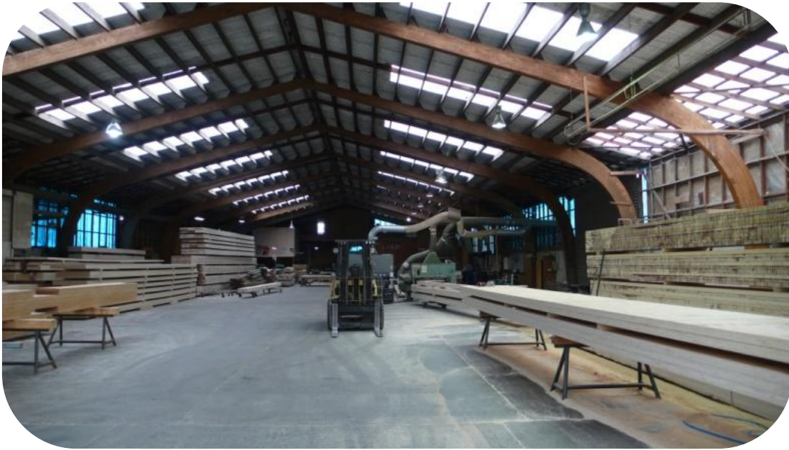
Figure E.1. Main fabricating area at HunterBond Ltd., near Nelson. LVL elements for the NMIT three storey Arts and Media Teaching block can be seen. Column – foreground left, Beam – foreground
