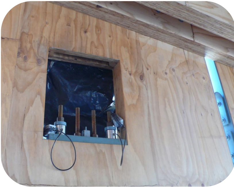
Figure E.17 Top of the shear wall showing top anchoring of Macalloy bars and instrumentation to measure movement in the Macalloy bars
