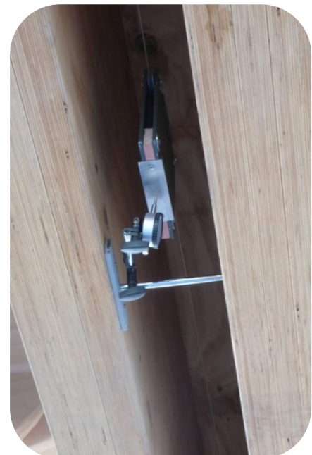
Figure E.38 Instrumentation to measure relative movement between LVL elements.
