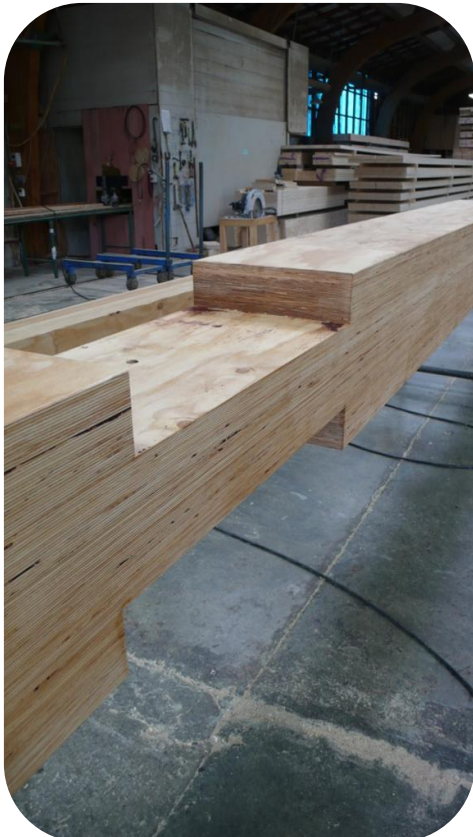
Figure E.3 LVL column showing check out to fit beams.
