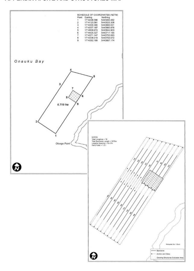
Figure 1. Copies of site map and structures plan showing location of new space and structures taken from Marlborough District Council coastal permit decision paper for U190782.
