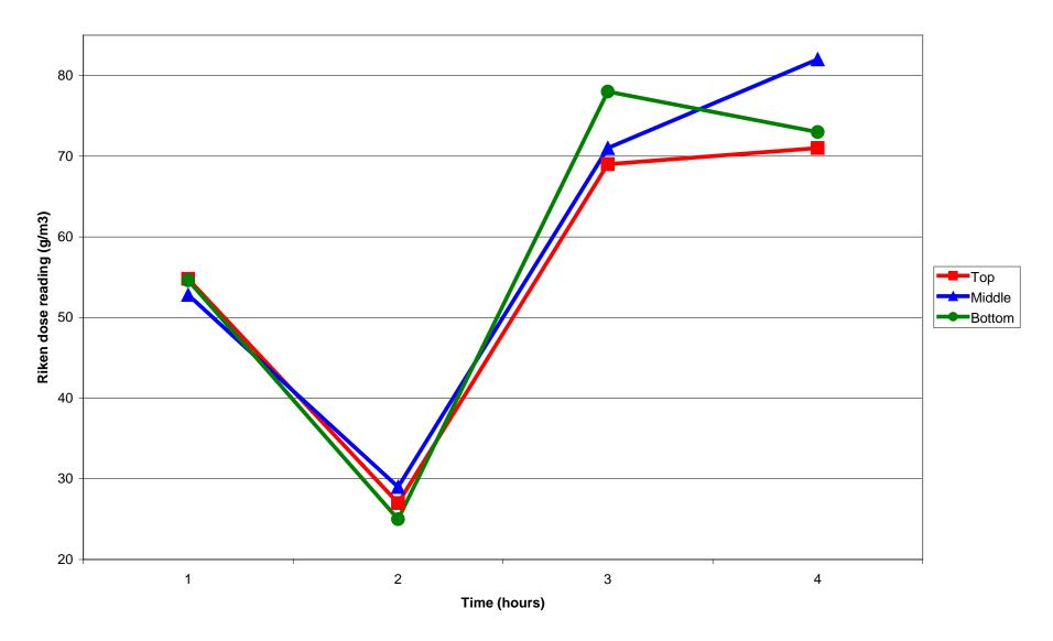
Figure 7: Comparison of fumigant levels at top, middle and bottom of RFR for first four hours following fumigation.
