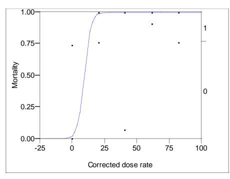
Figure 26: Logistic fit of *A. fulica* mortality vs. corrected methyl bromide fumigation dose rate at 30°Cel.
