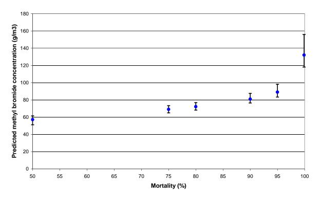
Figure 28: Inverse prediction from percentage mortality of *A. fulica* to provide methyl bromide fumigation dose rates at 17°Cel.
