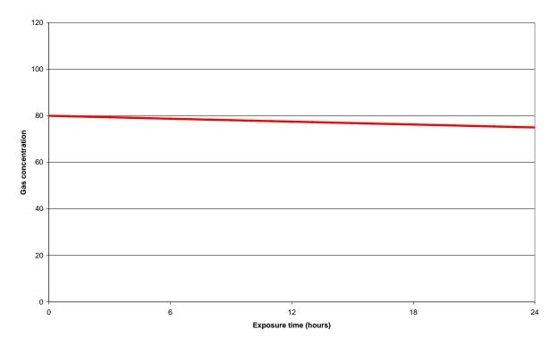
**Figure 10: Expected progressive gas concentrations with no loading on container.** Genera has suggested that a trial could be rapidly undertaken in New Zealand to confirm the fate of methyl bromide during fumigation. This would provide MPI with data on fumigant levels inside empty containers infected with an exotic organism.
