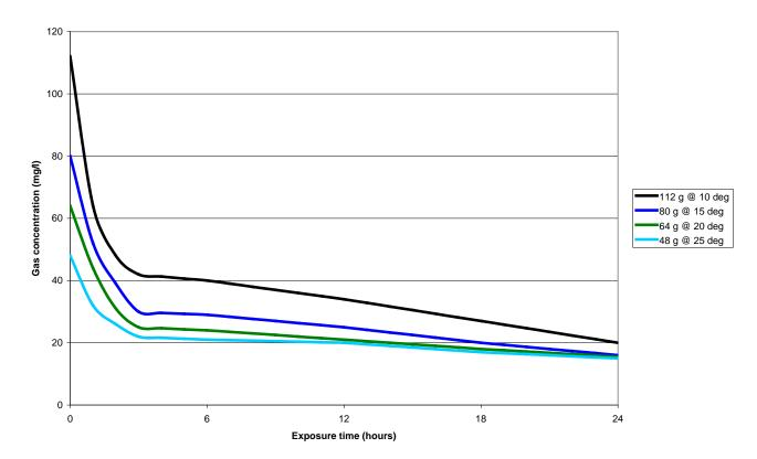
Figure 9: Theoretical progressive gas concentrations with 50% loading on container (based on Kawakami 2007).
