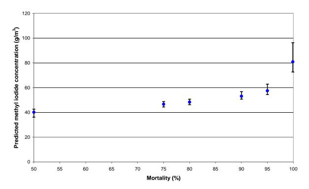
Figure 21: Inverse prediction from percentage mortality of *A. fulica* to provide methyl iodide fumigation dose rates at 17°Cel.
