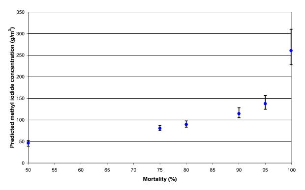
Figure 20: Inverse prediction from percentage mortality of *A. fulica* to provide methyl iodide fumigation dose rates at 12°Cel.
