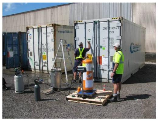
Figure 5: Fumigation equipment during Methyl iodide application.
