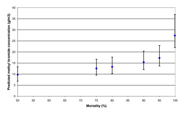
Figure 29: Inverse prediction from percentage mortality of *A. fulica* to provide methyl bromide fumigation dose rates at 30°Cel.
