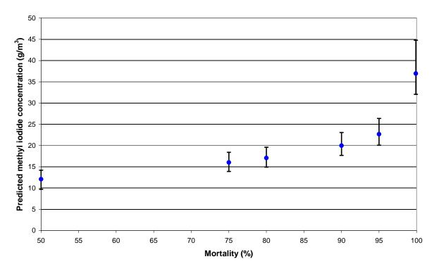
Figure 22: Inverse prediction from percentage mortality of *A. fulica* to provide methyl iodide fumigation dose rates at 30°Cel.
