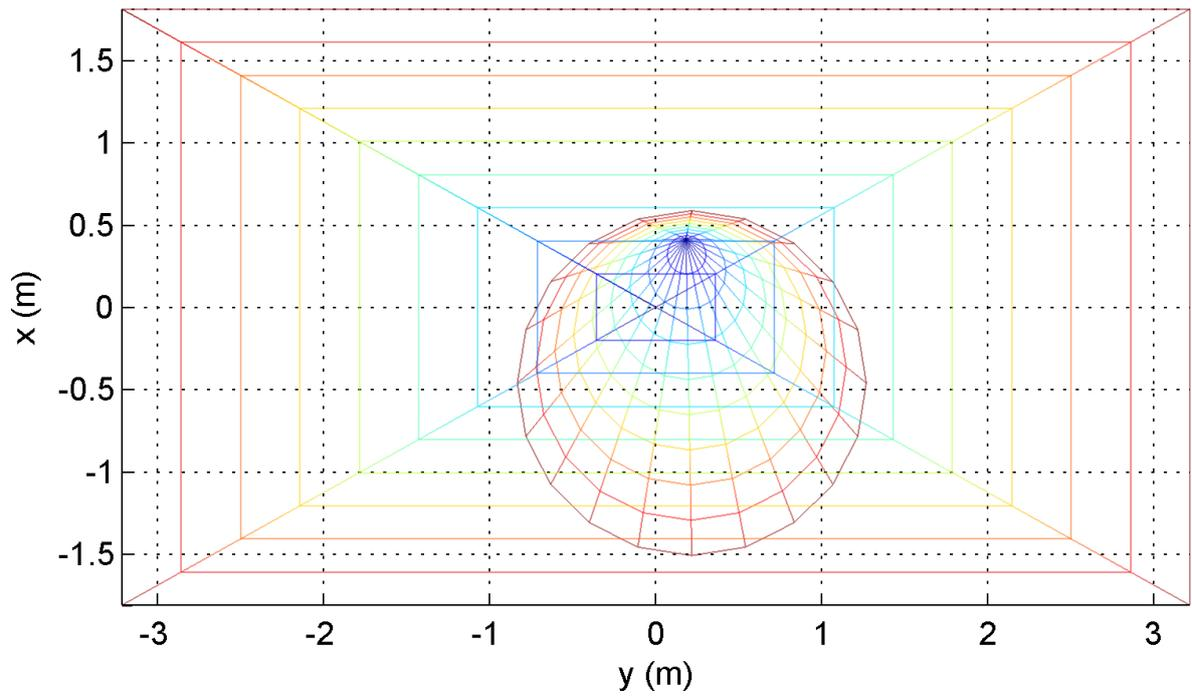
**Figure A2.2: Plot of the AOS alignment, where circles represent acoustic beam and squares video frame at different depth according to colours.**
