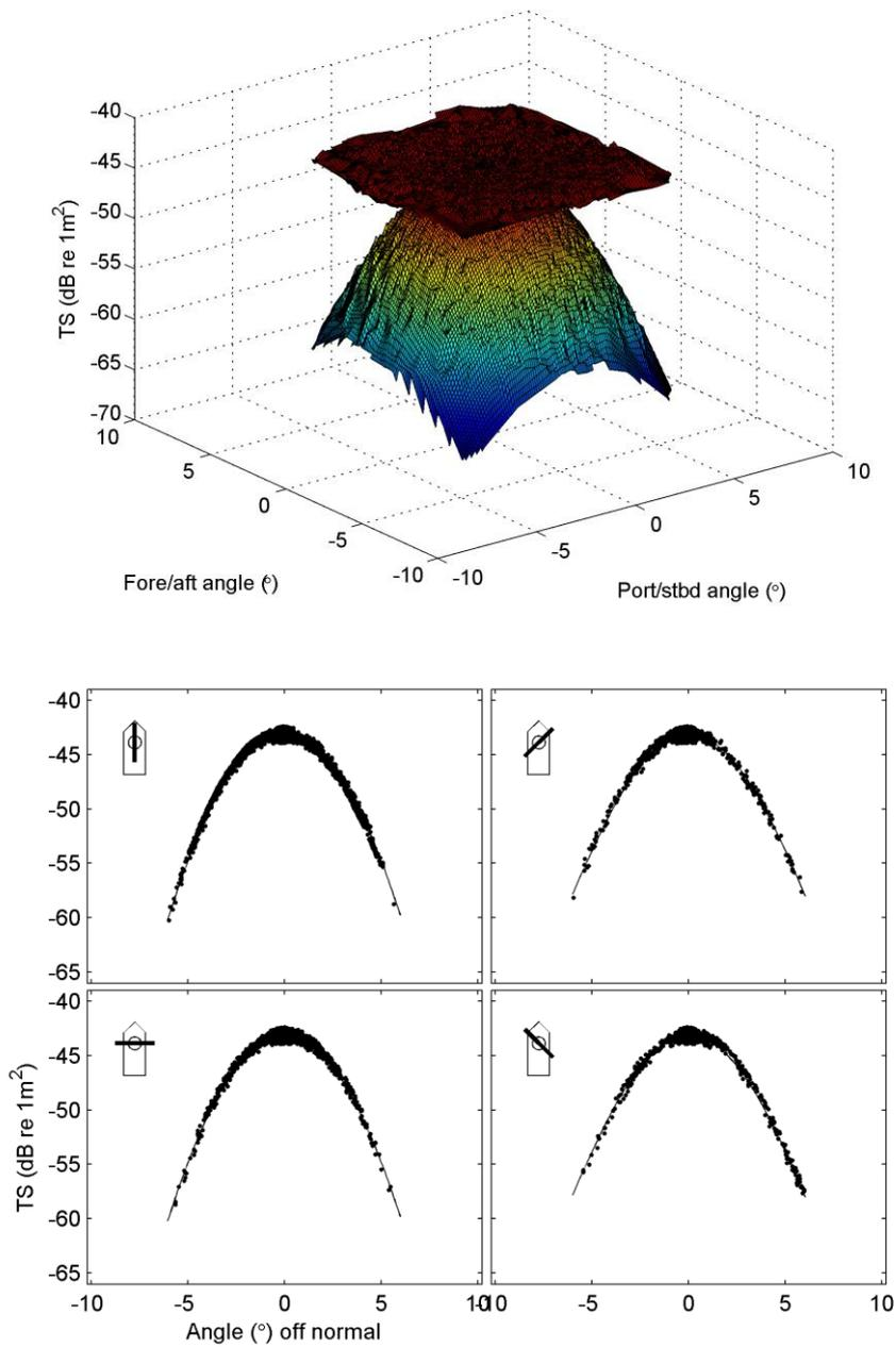
**Figure A2.1. The 38 kHz estimated 3D contour plot of the beam (a) from the sphere echo strength and position. Beam pattern results (b) from the 38 kHz analysis. The solid line is the ideal beam pattern fit to the sphere echoes for four slices through the beam.**
