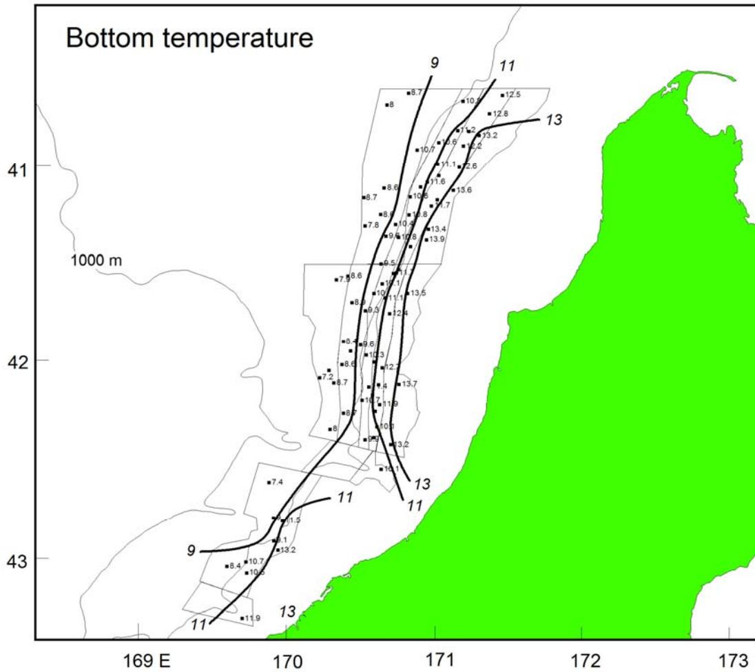
**Figure 39: Bottom water temperatures (°C) during the 2012 WCSI survey. Squares indicate bottom trawl tow positions. Not all temperatures are labelled where two or more tows were close together. Contours show isotherms estimated by eye.**
