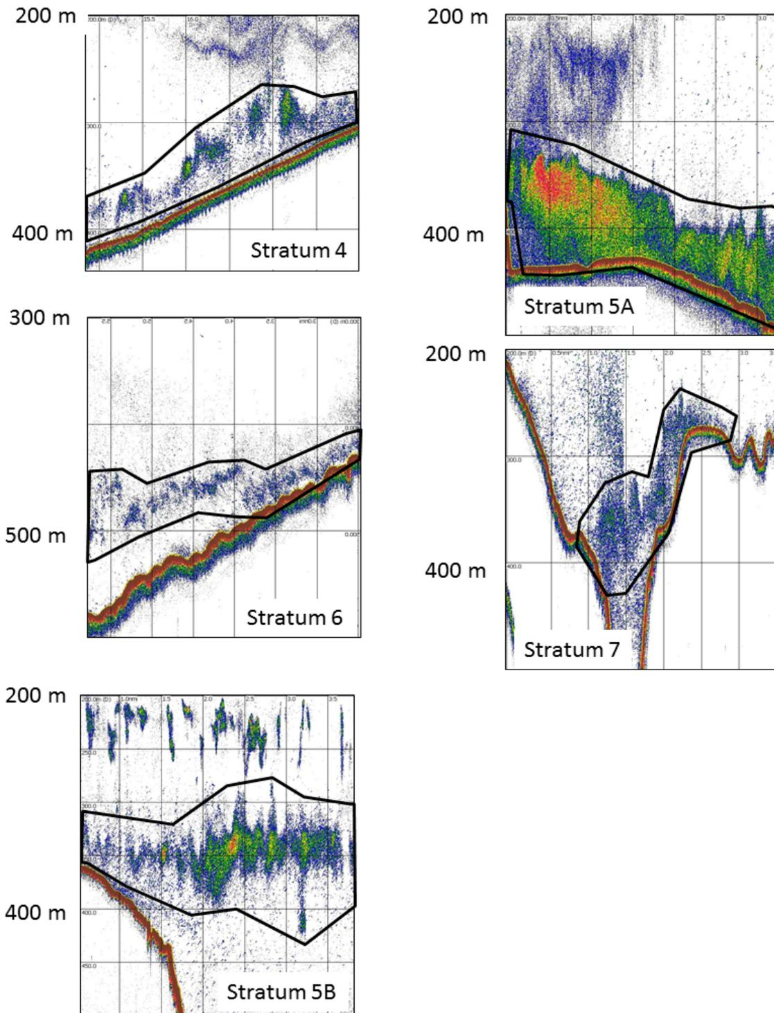
Figure 22: Examples of echograms showing hoki school marks by strata. Approximate boundaries of marks classified as hoki schools are shown by black boxes. Echograms are divided into cells of 50 m by 0.5 n. miles. Minimum echogram threshold is -70 dB.
