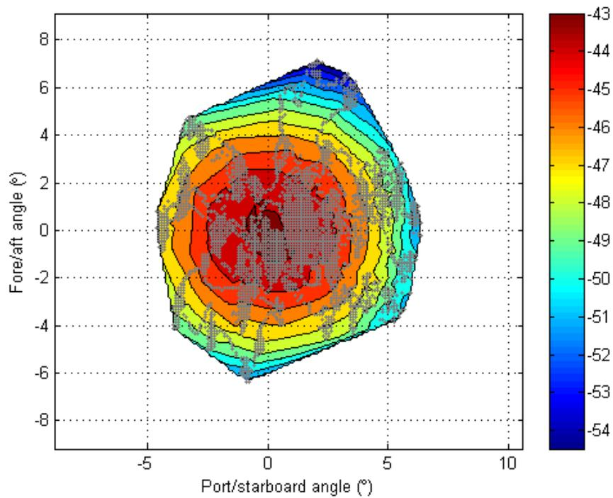
**Figure A1.1.** The 18 kHz estimated beam pattern from the sphere echo strength and position. The '+' symbols indicate where sphere echoes were received. The colours indicate the received sphere echo strength in dB re 1 m<sup>2</sup>.
