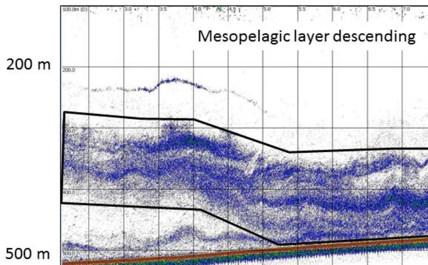
Figure 24: Examples of an echogram from stratum 1&2 showing mesopelagic layers descending at dawn. The approximate boundary of the mark is shown by the black box. Echogram is divided into cells of 50 m by 0.5 n. miles. Minimum echogram threshold is -70 dB.
