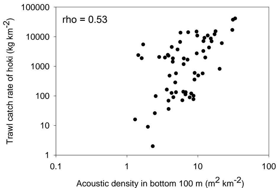
Figure 26: Relationship between trawl catch rate of hoki and bottom-referenced acoustic backscatter recorded during bottom tows during the 2012 WCSI survey. Rho value is Spearman's rank correlation coefficient.
