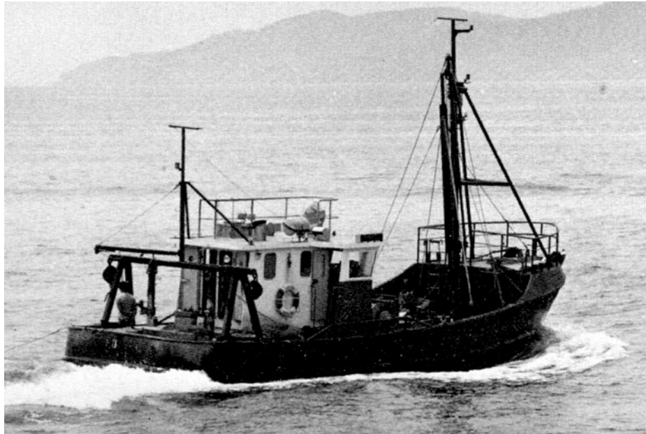
Figure 22: Eskdale , a 17 m steel vessel typical of the trawler-seiners built in the late 1960s and 1970s. From Paul (1977).
