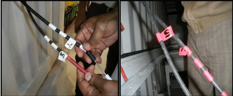
Numbering system to differentiate the house probes in the chamber (white tapes for the right chamber and red tapes for the left chamber). Numbers on the tapes refer to the probe numbers.
