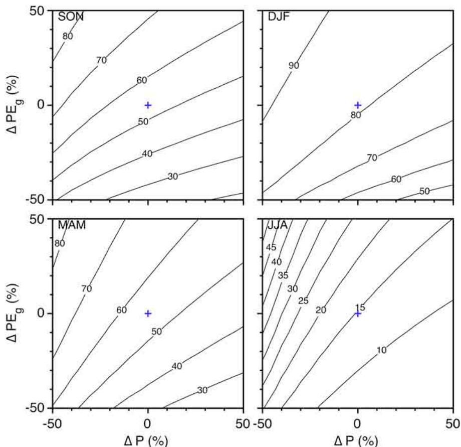
**Figure 11.** Response surface representations of the sensitivity of seasonal mean SWD (mm, isopleths) to conjoint change in P and  $PE_g$ . The '+' symbols denote the results for the DWBM run for unadjusted P and  $PE_g$  (1932-2007). Baseline run parameter values.
