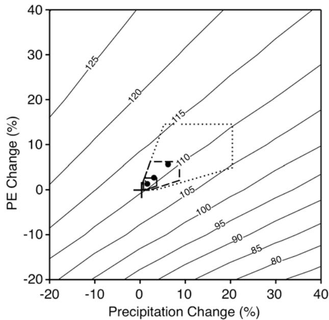
**Figure 1.** Example response surface, showing the sensitivity of mean summer soil water deficit (isopleths in mm) for an Auckland site to conjoint changes in precipitation and potential evaporation (PE). Superimposed on the response surface are climate change scenario best estimates (dots) and uncertainty envelopes for 2020, 2050, and 2100. Modified after Fowler (1999).
