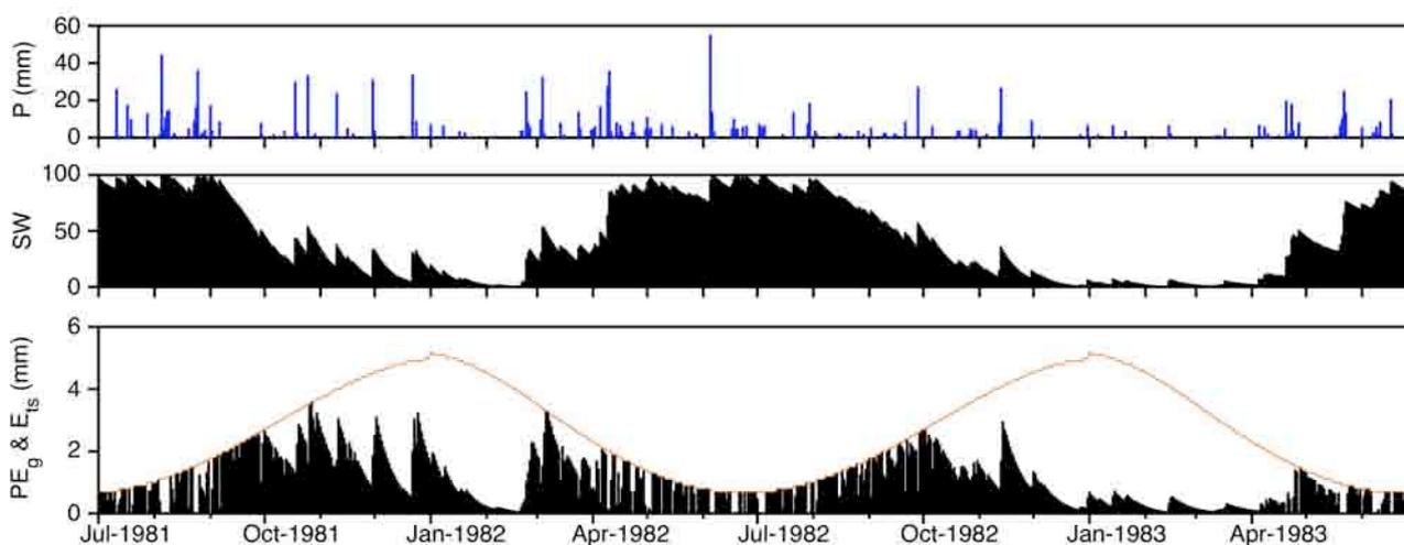
**Figure 9.** DWBM daily simulation results (July 1981 to June 1983). Top: daily precipitation ( $P$ ). Middle: soil water content (SW). Bottom: climatological potential evaporation ( $PE_g$ , thin line) and actual evaporation excluding interception ( $E_{ts}$ , bars).
