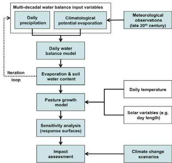
**Figure 2.** Research framework for analysis at a single site. White boxes represent components that are not implemented in the pilot study. The iteration loop refers to multiple runs of the DWBM with incremental adjustments to precipitation and potential evaporation, required to produce the sensitivity analysis response surfaces.
