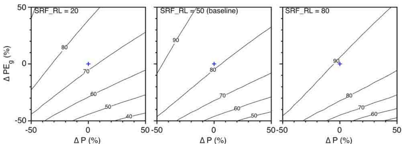
**Figure 12.** Sensitivity of DJF mean SWD (mm, isopleths) to conjoint change in P and PE<sub>g</sub>, for alternative values for SRF\_RL (other parameters set to baseline values). The '+' symbols denote the results for the DWBM run for unadjusted P and PE<sub>g</sub> (1932-2007).
