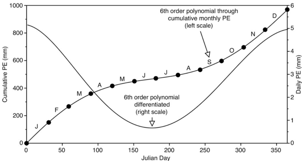
**Figure 8.** Calculation of climatological PE values from monthly mean PE for Napier. Monthly PE data from NZMS (1986).
