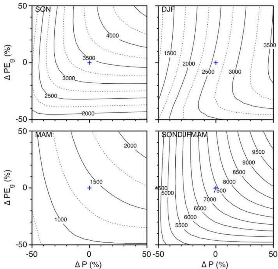
**Figure 15.** Sensitivity of seasonal mean pasture productivity (DM kg/ha) to conjoint change in P and  $PE_g$ . The '+' symbols denote the results for the DWBM run for unadjusted P and  $PE_g$  (1932-2007). AWC = 200mm. Baseline run values for other parameters.
