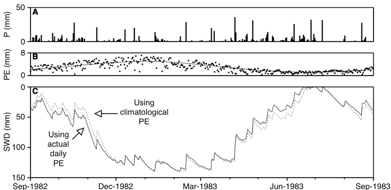
**Figure 4.** Comparison of DWBM simulation results (Sept-1982 – Aug-1983) using actual and climatological PE estimates. (A) Daily rainfall input common to both model runs. (B) Actual daily PE (dots) and climatological PE (curve) used as input to the two DWBM simulations. (C) Modelled soil water deficit (SWD). Results are for Auckland pasture. Note that this is the *worst* result obtained for 13 simulation years. Modified after Fowler and Adams (2004).
