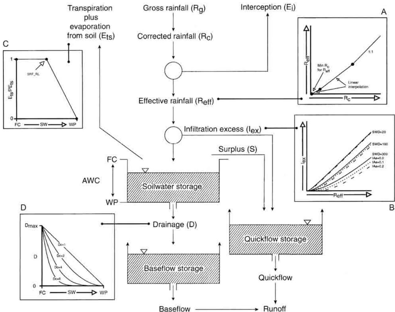
**Figure A1.** Schematic representation of the DWBM. Source: Fowler (1999).
