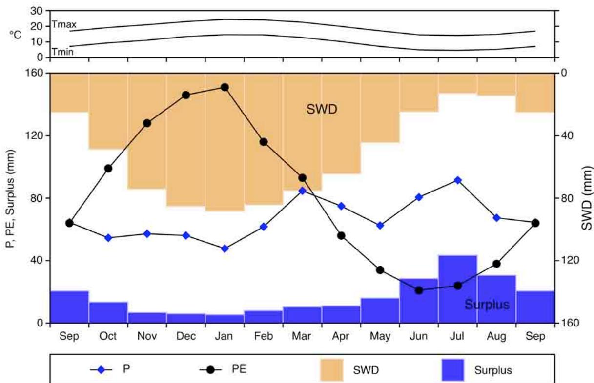
**Figure 6.** Napier hydroclimatology. Top: monthly mean minimum and maximum surface air temperatures (Tmin, Tmax) for Nelson Park (1971–2000). Bottom: monthly mean P and PE for Nelson Park (1941–1984) and DWBM-simulated soil water deficit (SWD) and surplus for a soil with an AWC of 100 mm. Sources: Nelson Park data from the National Climate Database (cliflo.niwa.co.nz) and NZMS (1986).
