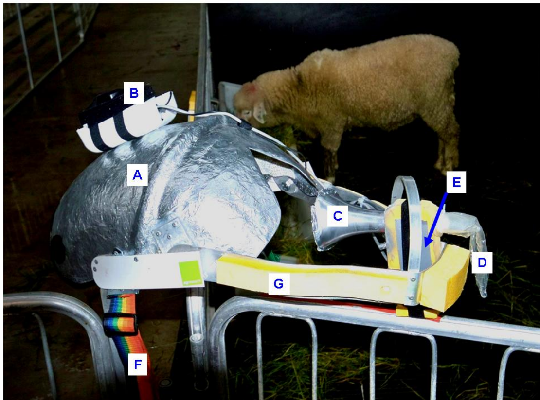
Plate 2: Close-up of urine sensor apparatus (resting on steel gates). A – fibreglass mould to locate urine sensor on rear of sheep; B - electronics box containing batteries, RI sensor control and GPS circuitry - a GPS antenna is located on top of this box; C - funnel through which urine passes; D - condom for collecting urine sample (for validation work only); E - The RI sensor is contained within a foam block to provide protection and to exclude sunlight; F - one of 3 straps that holds apparatus on the sheep; G – adjustable aluminium hoop with rubber protection to hold urine sensor in position. As the sheep squats to urinate the apparatus pivots about the hind leg joints such that urine passes into funnel.
