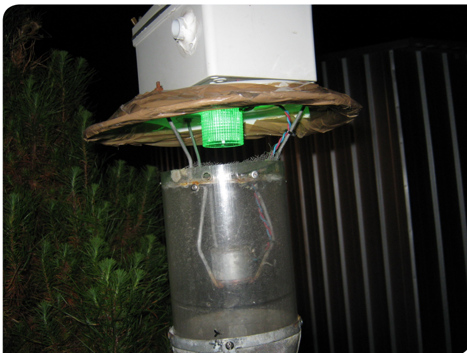
Figure 2: Typical green LED light trap with suction fan that draws insects into a jar of ethanol at the base of the trap. Photo: Peter Goldsbury, AsureQuality
