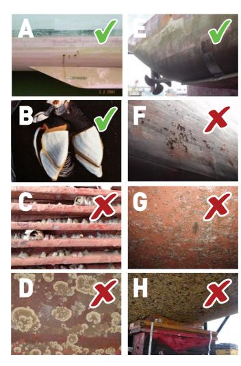
The only fouling a long-stay vessel may have is a slime layer (A) and gooseneck barnacles (B). Any other species, such as the acorn barnacle (C), or bryozoans (D), are not allowed. The images on the right show a slime layer (E) which would meet the new requirements, and moderate (F) extensive (G) and very heavy (H) levels of fouling which would not meet the new requirements. (Images: John A Lewis, ES Link Services Pty Ltd).
